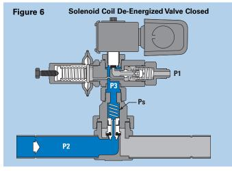
bleeds through the piston to the chamber above the piston. However, since the hot gas cannot bleed through the pilot valve, the pressure on top of the main piston (P3) increases, driving the piston down and closing the main port.
