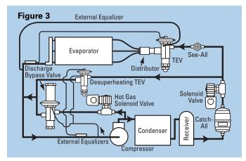
(Figures 1 and 3), require externally equalized valves, this model will be the most readily available one in the field. Therefore, it is suggested that in all cases, the externally equalized DBV be applied.
