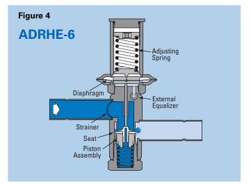
evaporator temperature change from closed position to rated opening. A 6°F change is considered normal for most applications and is the basis of our capacity ratings. Multipliers for other temperature changes are given in the Selection Procedures section.
